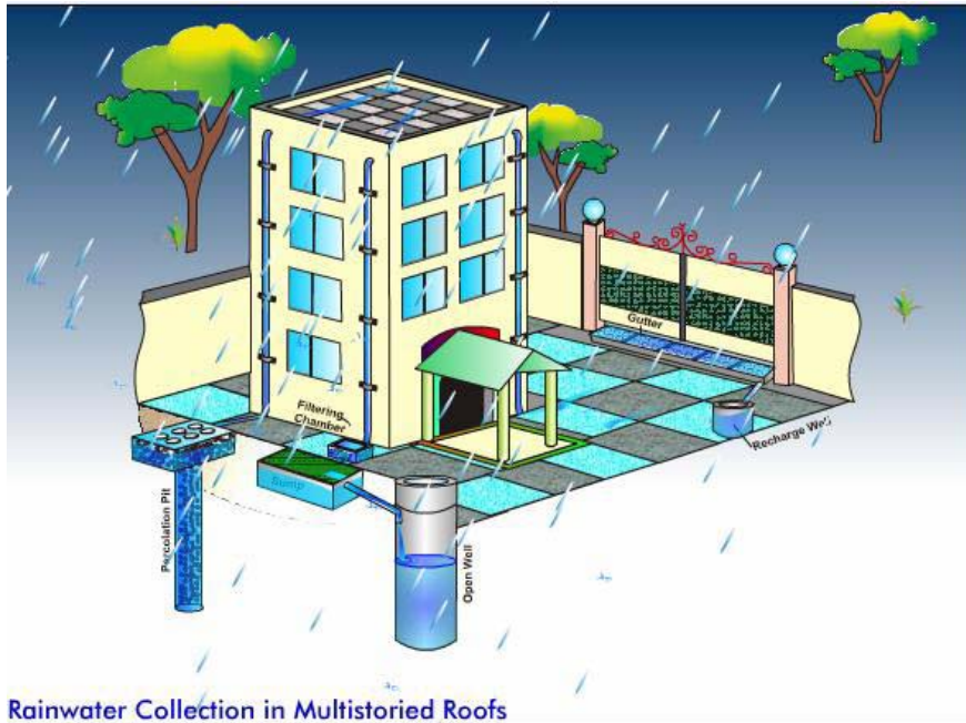
Rainwater Collection in Multistoried Roofs
